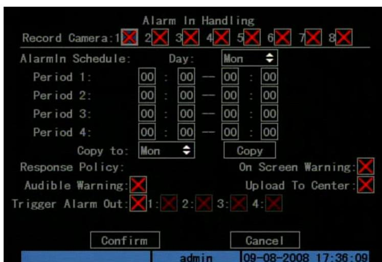
Fig. 5.24 Alarm in handling setup
